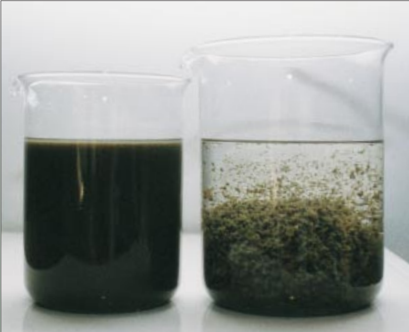
Sludge conditioning with polyelectrolyte
